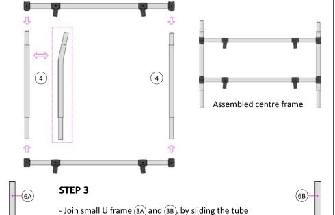
connector (7) inside the frames until the screw holes align.
